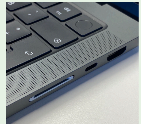
Figure 1: BaseQI USHII-420A with an 1 TB microSD Card inside in a MacBook Pro 14". The microSD is inside the SD card slot.
