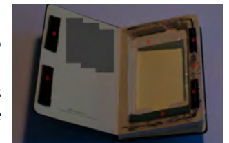
a: Velcro, b: foam to press the iPod into the casing, c: opening for the on/off button, d: thread that keeps the pages together and the Velcro, e: plastic foil to protect the paper; the complete inside of the hole in the pages is covered with glue
